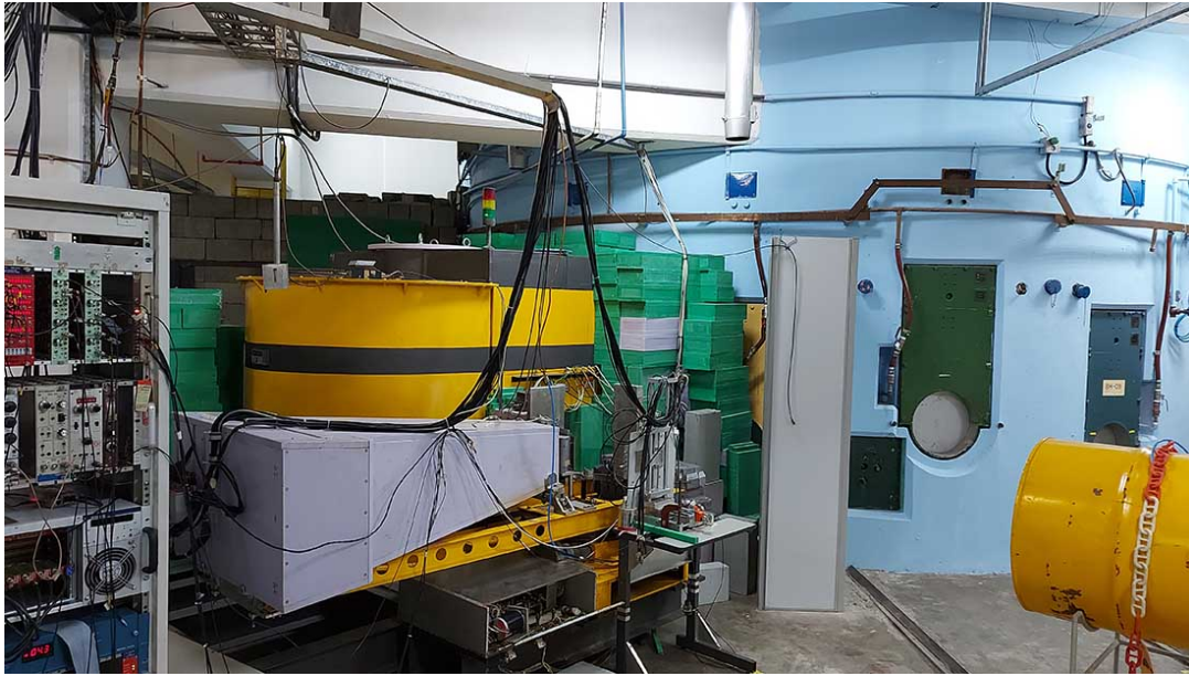
Figure 5.20: The blue wall is the reactor pool wall, where it is possible to see two closed beam port doors. The yellow structure encases the AURORA experiment's monochromator and two focusing structures; the set allows the desired neutron energy to be selected. The violet structure contains the position-sensitive detectors of the AURORA experiment [89]. The electronics rack is also visible on the left and the beam stopper (yellow barrel) on the right.
