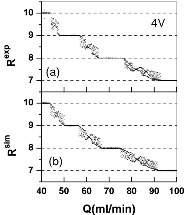
FIG. 4: (a) Experimental bifurcation diagram for  $4V$  sound wave amplitude. (b) Simulation with  $A = 1.42 \times 10^{-3}$ ,  $V_c = 0.0634$  and  $\beta = 0.415$ . In addition to the experimental frequency lockings well reproduced for  $k=\text{integer}$  and for  $k=\text{half integers}$  we can observe period 3 for  $k=22/3$  and  $k=23/3$ .
