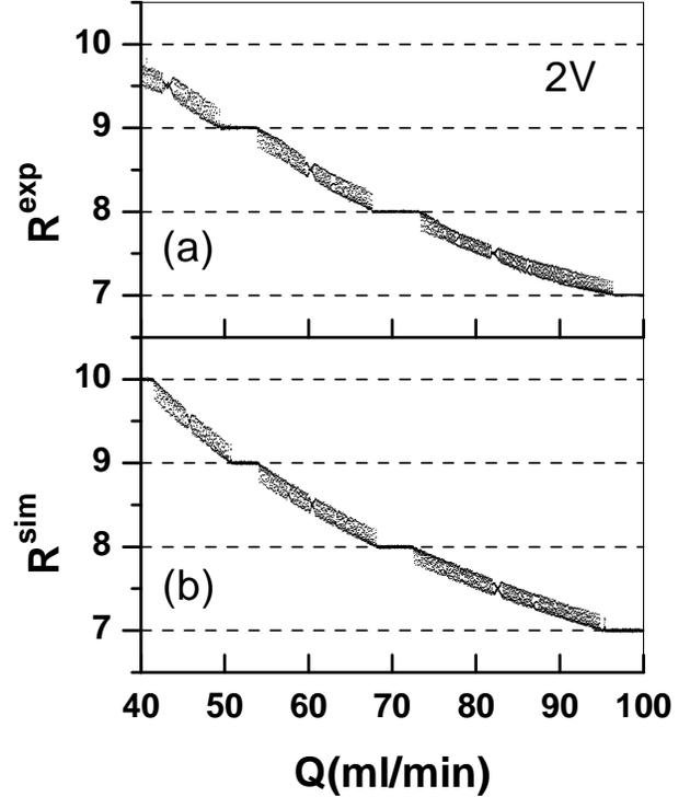
FIG. 3: (a) Experimental bifurcation diagram for  $2V$  sound wave amplitude. (b) Simulation with  $A = 0.75 \times 10^{-3}$ ,  $V_c = 0.0631$  and  $\beta = 0.40$ . The experimental frequency lockings are well reproduced for  $k$ =integer numbers as well as for  $k$ =half integers.
