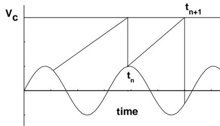
FIG. 1: The integrate and fire dynamics model with the sinusoidal bubbles initial conditions drive by the sound wave.
