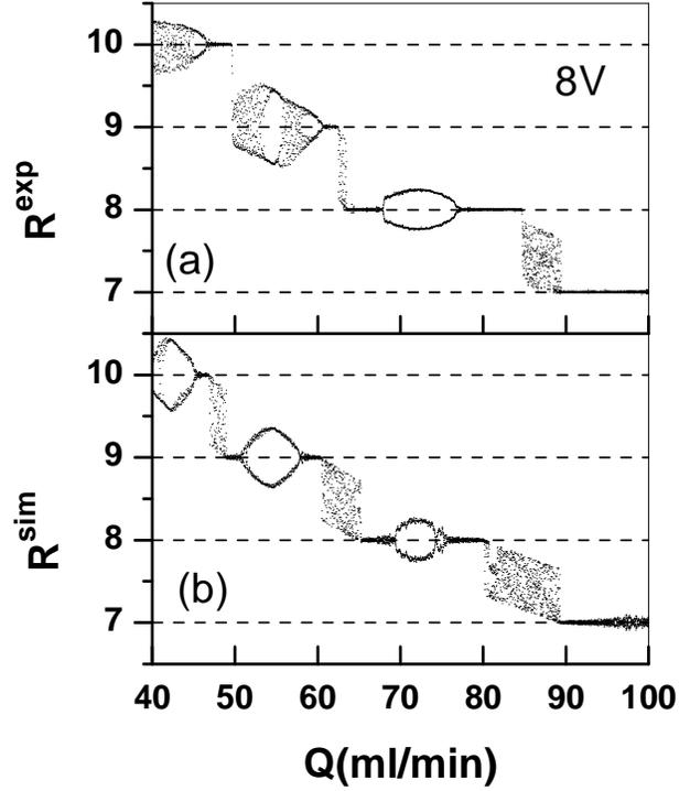
FIG. 6: (a) Experimental bifurcation diagram for 8V sound wave amplitude. (b) Simulation with  $A = 2.8 \times 10^{-3}$ ,  $V_c = 0.064$  and  $\beta = 0.416$ . We can see chaotic behavior related to the doubling period in each branch of period 2.
