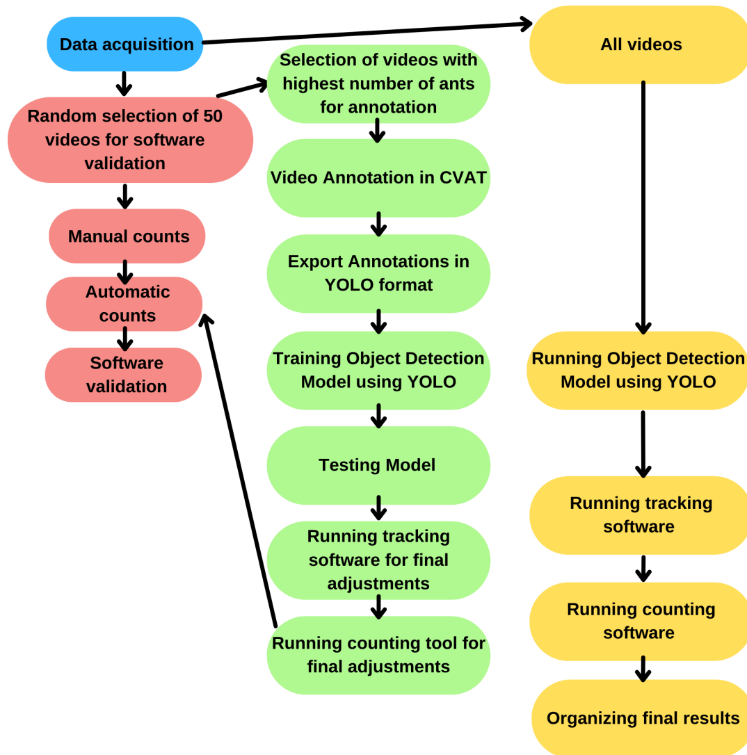
Figure 1: Flowchart of all the steps involved in our video-tracking software development. Blue box involves data acquisition (experiments). Red boxes show all steps involved in the software validation stage. Green and yellow boxes show respectively the deep learning train model stage and running our model.
