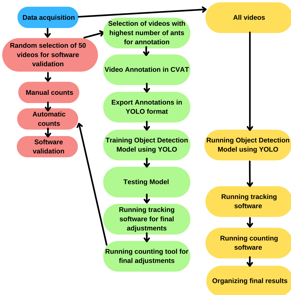
Figure 5) Flowchart of all the steps involved in our video-tracking software development. Blue box involves data acquisition (experiments). Red boxes show all steps involved in the software validation stage. Green and yellow boxes show the deep learning train model stage and run our model results for all our data.
