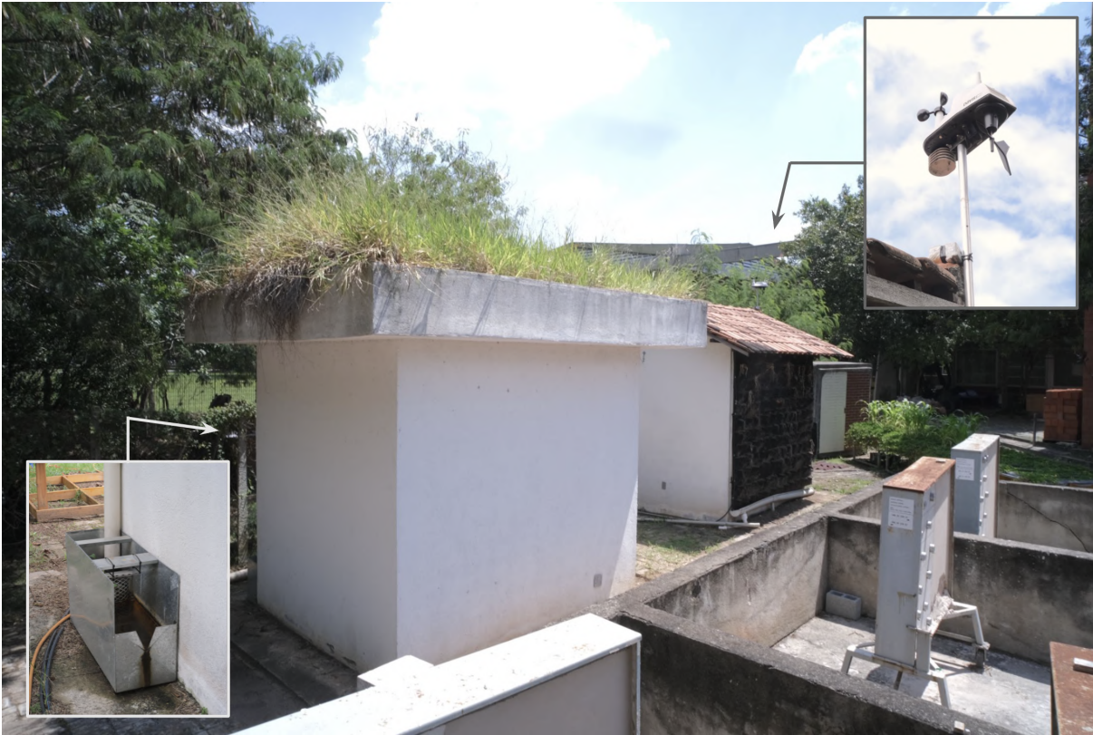
Figure 24 – Vegetated roof building prototype and ceramic tiled roof building prototype, triangular-notch weir tank with ultrasonic sensor and Vantage Vue weather station.
