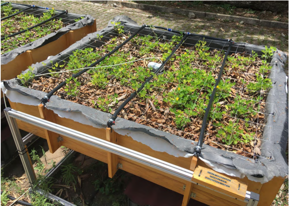
Figure 41 – Final testbed with the grid for point-intercept method.
