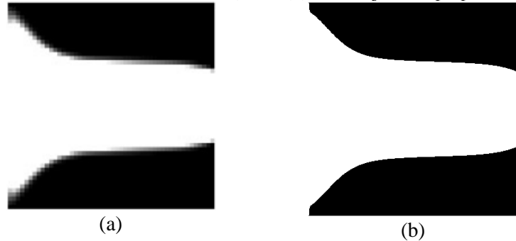
Figure 17. Optimized converging nozzle under laminar incompressible regime reported by (a) literature (Borrvall and Petersson 2003) and (b) the “adjointTopOptFoam” software
