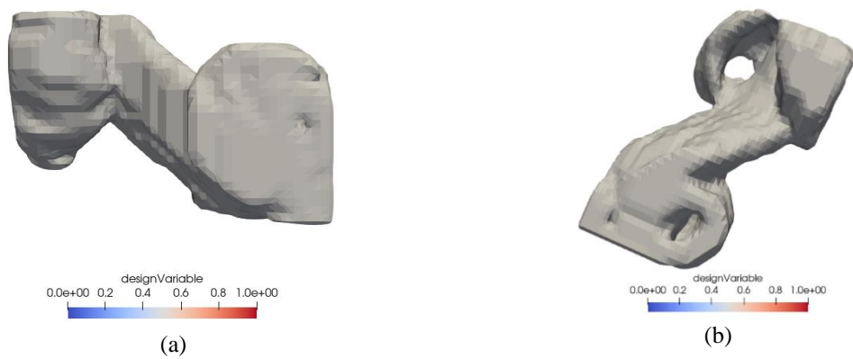
Figure 38. Optimized container under the IDV approach: (a) side and (b) superior view
