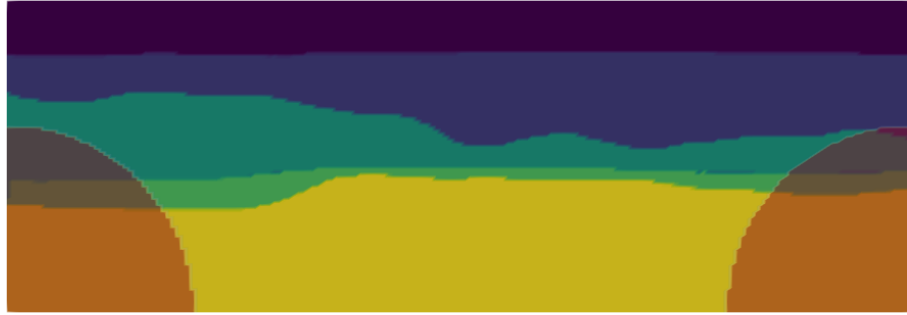
(a) Reference velocity model with shadow region \Omega_s marked. The corners are occupied by quarter circles with 3 km radius.
