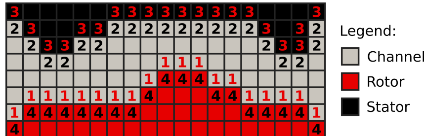
Figure 2.8 – Illustration of active elements during the optimization of a labyrinth seal. (1) Fluid elements that can change to rotor; (2) fluid elements that can change to stator; (3) stator elements that can change to fluid; (4) rotor elements that can change to fluid. Elements with black numbers are active during stator expansion/rotor contraction and elements with red numbers are active during rotor expansion/stator contraction.
