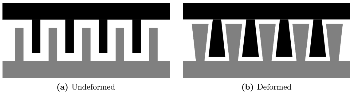
Figure 1.4 – Concept of an inflatable labyrinth seal. The undeformed state can be assembled and the deformed state offers higher leakage reduction.
