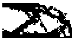
(b) Added connectivity criteria to the objective function with a small weighting coefficient
