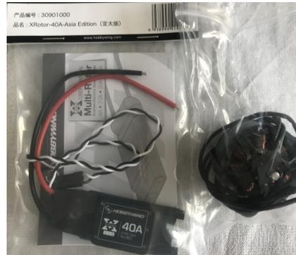
(b) Motor Modelo MN3508 KV580 e ESC XRotor-40A.
