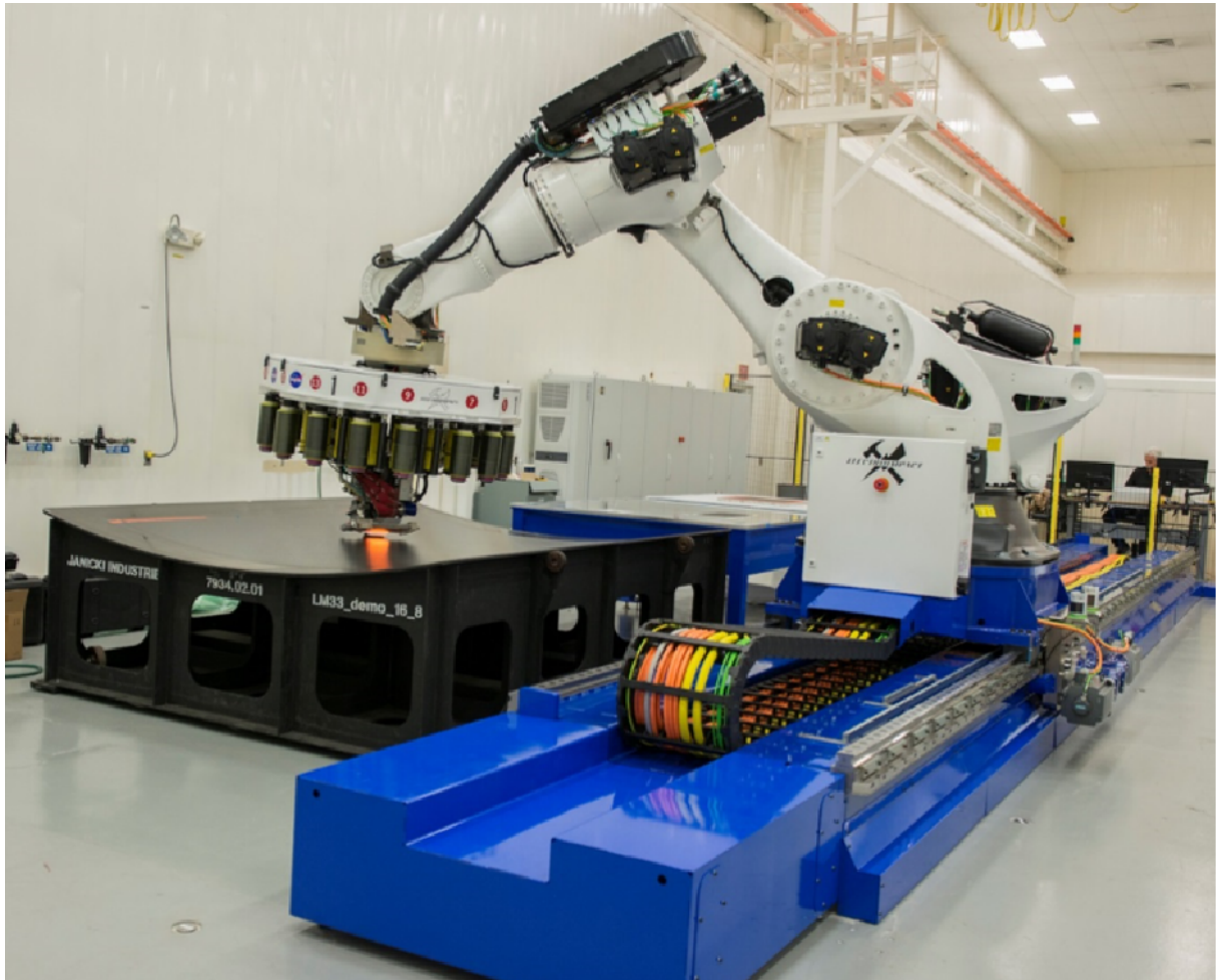
Figura 1.2 – Braço robótico para manufatura aditiva de materiais reforçados com fibra de carbono. Retirado de: https://www.nasa.gov/centers/marshall/news/news/releases/2015/robotic-manufacturing-system-will-build-biggest-composite-rocket-parts-ever-made.html
