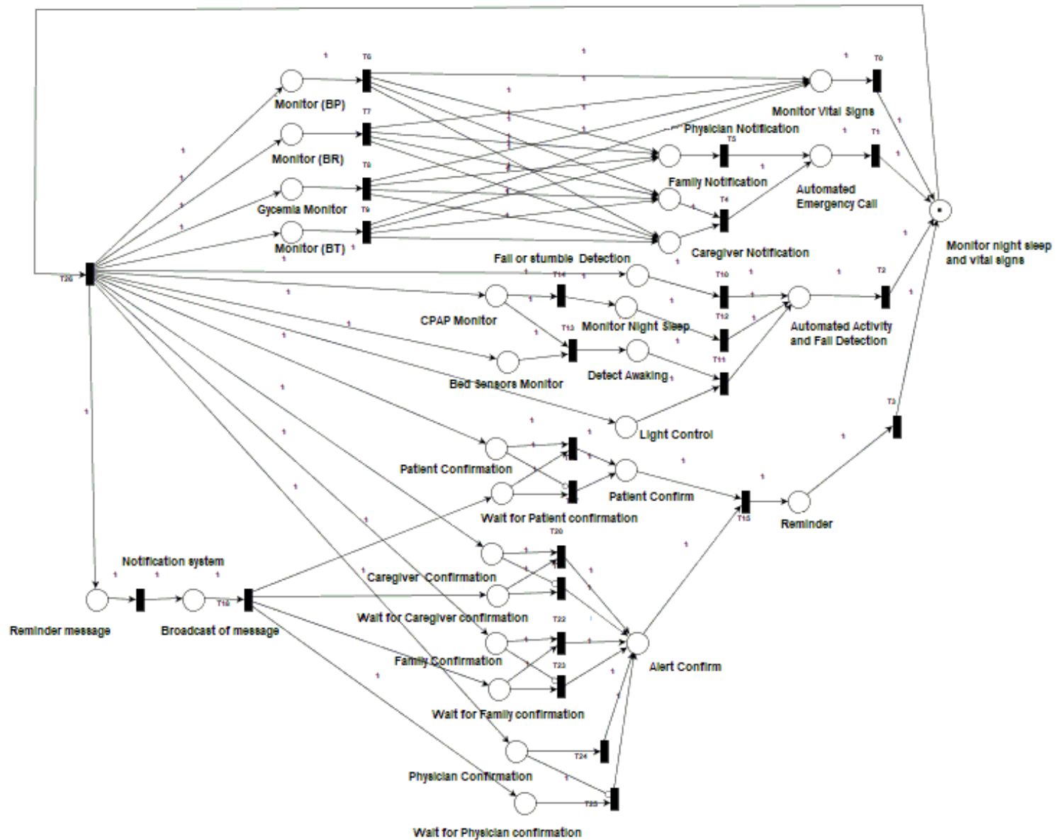
Figure 26 – Petri net for Monitor elderly night sleep and vital signs ("System To-Be").
