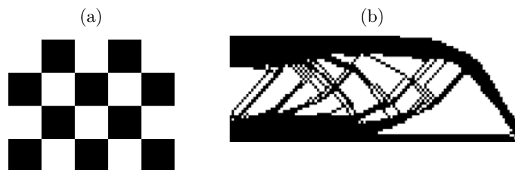
Figure 9: (a) The checkerboard pattern and (b) a typical topology with checkerboard pattern.
