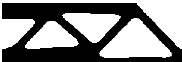
Figure 16: BESO characteristic result with well-defined boundary.
