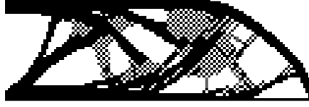
Figure 19: Mesh dependency problem: different topologies given by different discretizations.
