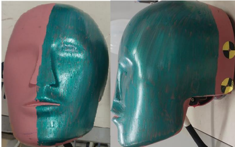
Figure 26 – Front and side view of dummy's head with grease paint applied to the side that is expected to be in contact with the airbag (Erikson and Piroti, 2018).
