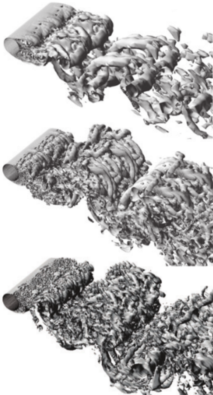
Figure 5.3: Increasing levels of refinement from top to bottom, accentuating DES tendency toward DNS with shortening of cell sizes. Adapted from Spalart (2009).
