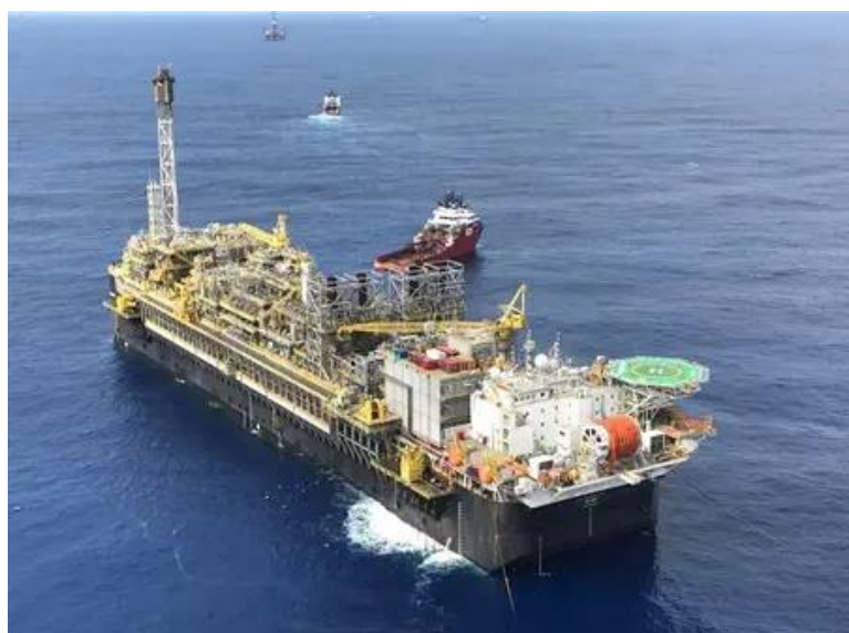
Figure 1-3: Ship-Shaped FPSO example
