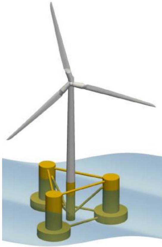
Figure 2.5: NREL DeepCwind floating wind system design [44].
