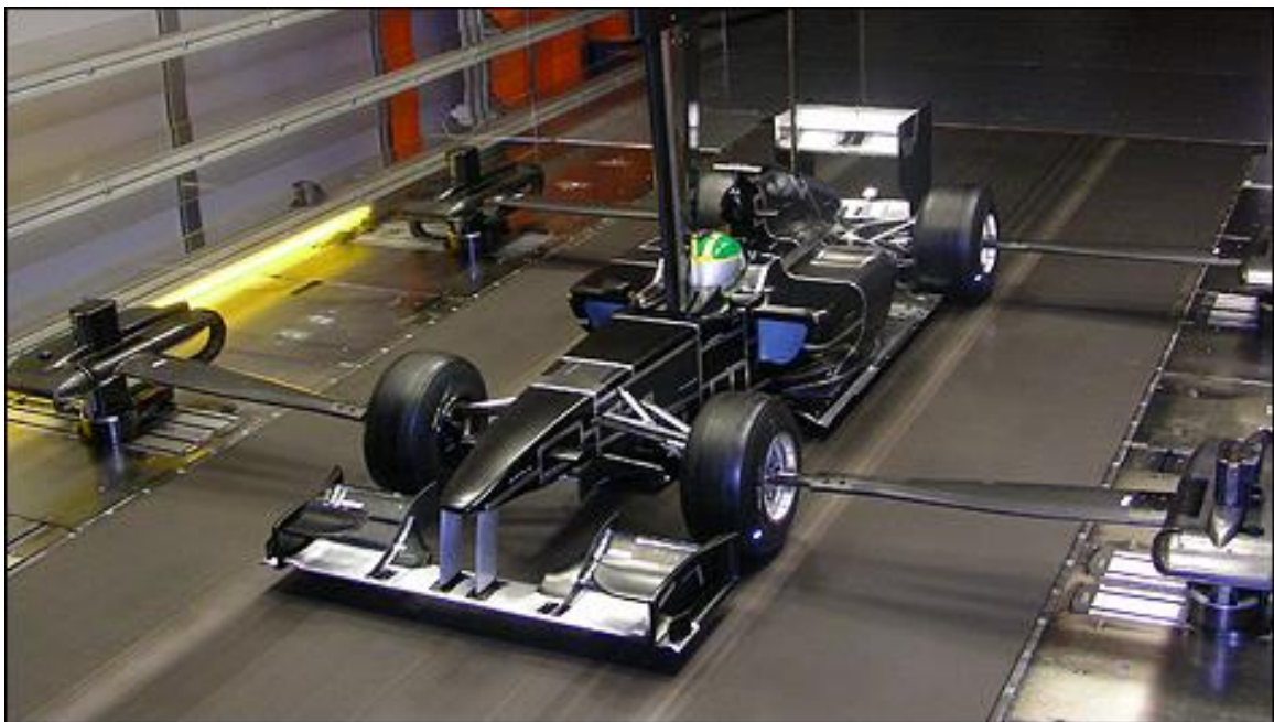
Figure 1-13 The model race car being tested in the wind tunnel (Katz, 2006).
