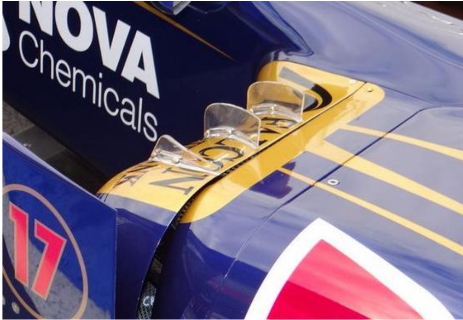
Figure 1-8 The vortex generators found on Toro Rosso F1 cars ( https://www.carthrottle.com/post/vortex-generators-how-do-they-work/ ).
