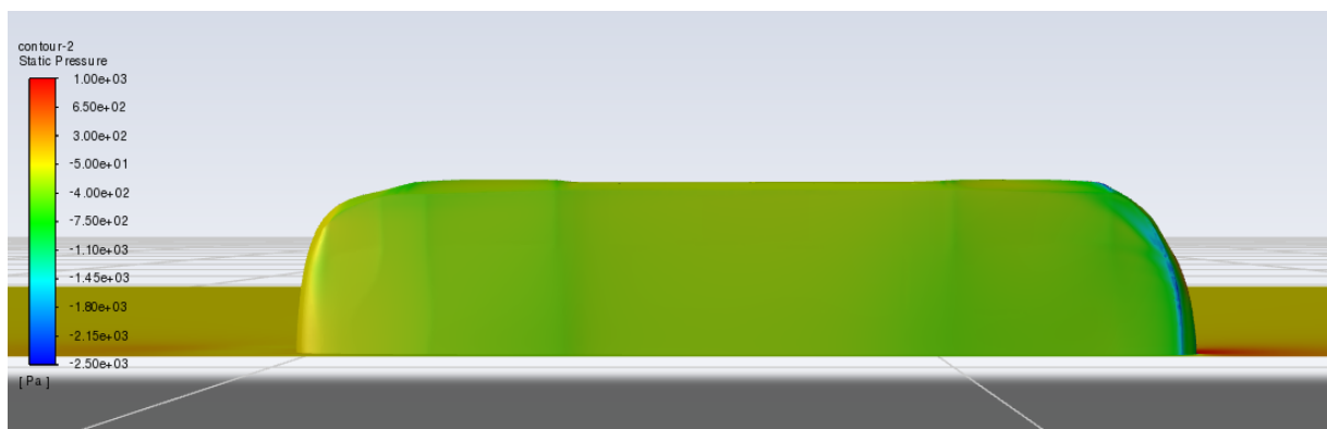
Figure 4-51 Contours of static pressure of the car original geometry bottom surface.
