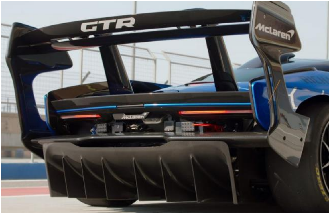
Figure 1-9 McLaren Senna GTR rear Diffuser (automais.autosport.pt).
