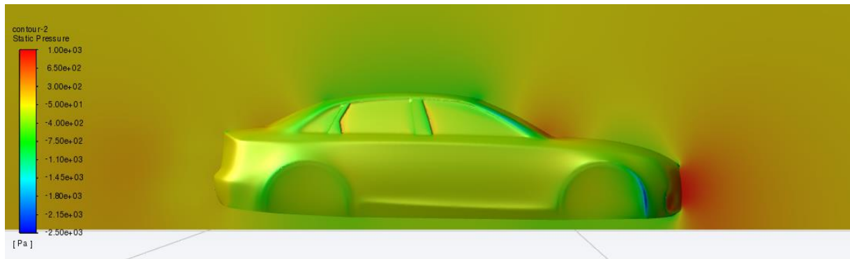
Figure 4-49 Contours of static pressure of the car original geometry.
