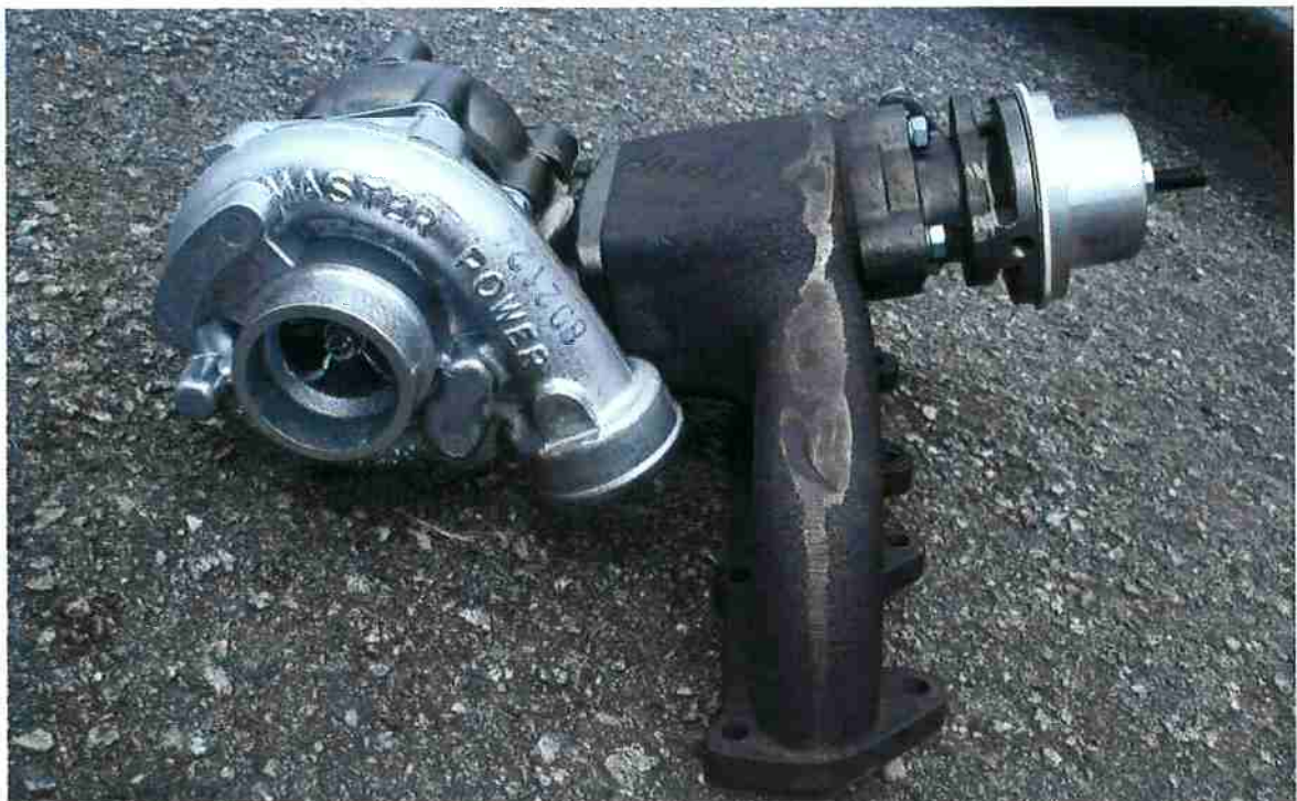
Fig. 10 – Coletor de escape com turbocompressor e wastegate
