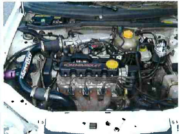
Fig. 31 – Motor com turbocompressor
