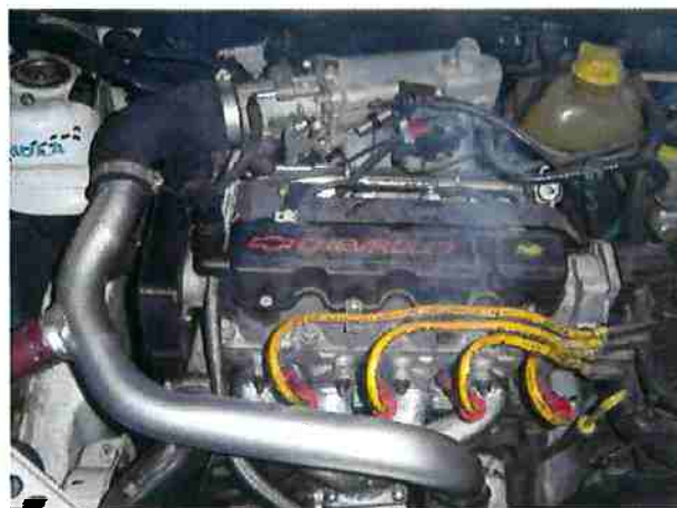
Fig. 28 – Motor com turbocompressor
