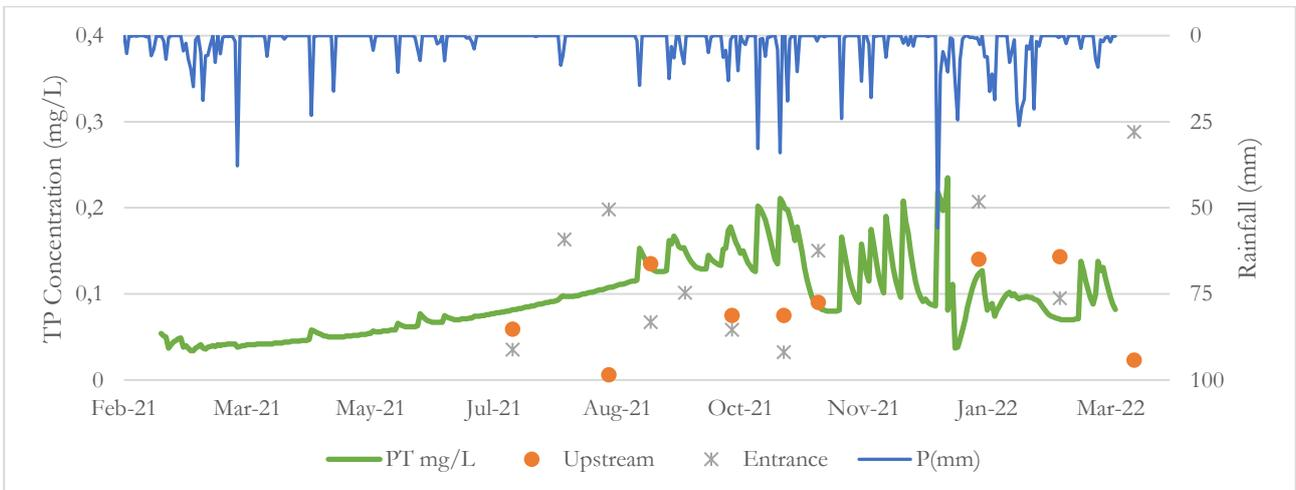
Figure 86 - TP Concentrations [mg/L] for Hedberg Reservoir – simulated (green line) and observed (dots)
