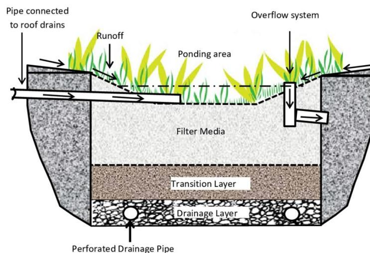
Figure 22 - Schematic of a Section View of a Bioretention Area
