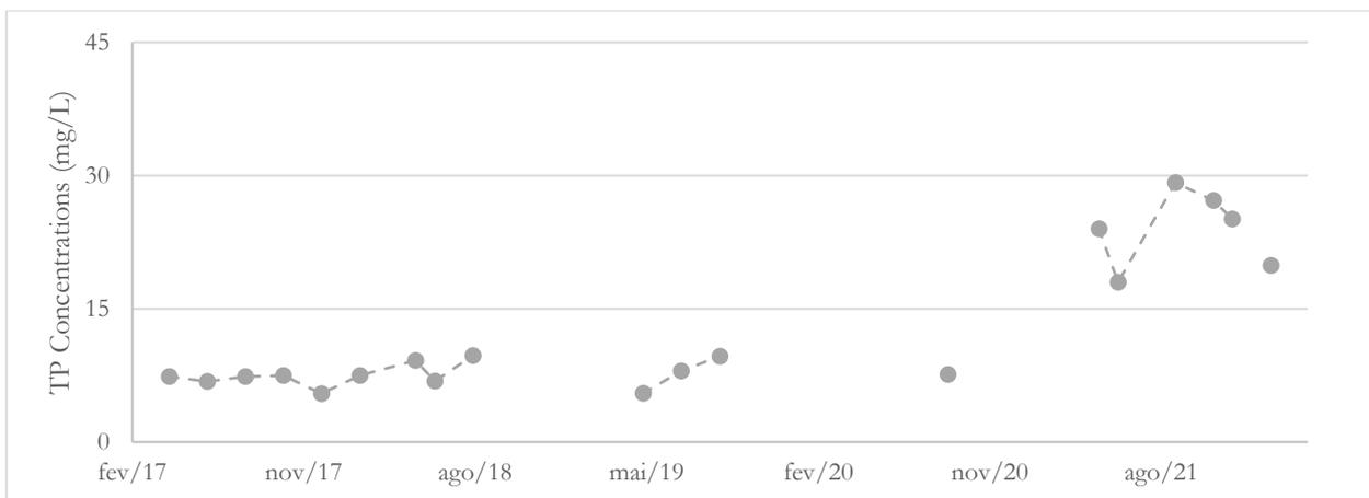
Figure 37 – Total Phosphorus released by WWTP Ipaneminha
