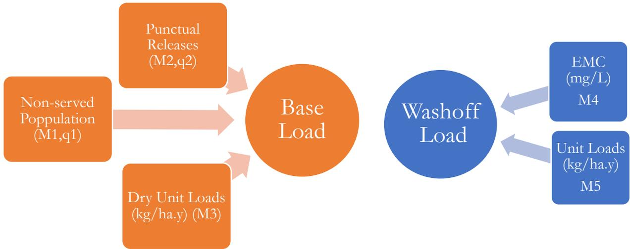
Figure 64- Load Model in CAbc Qual
