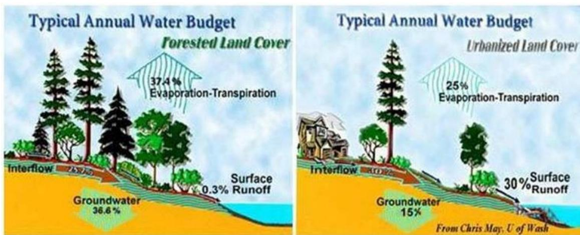
Figure 8 - Water balance for forested (left) and urban watersheds (right)
