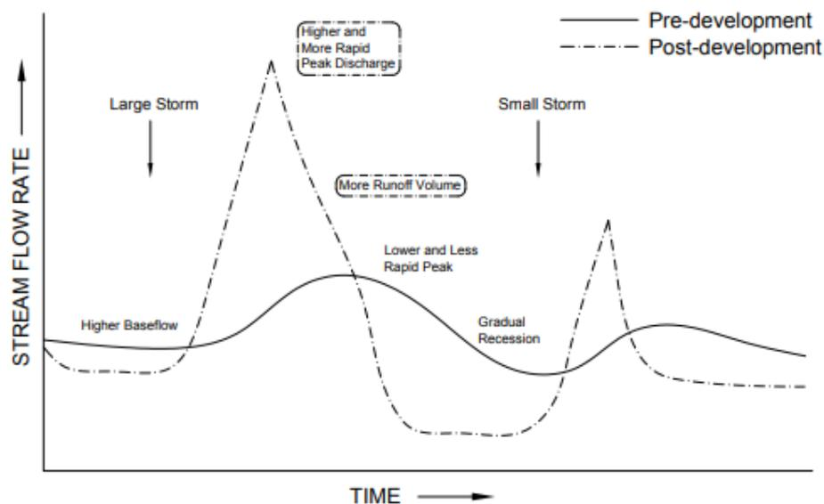
Figure 9 - Hydrograph under Pre- and Post-Development Conditions
