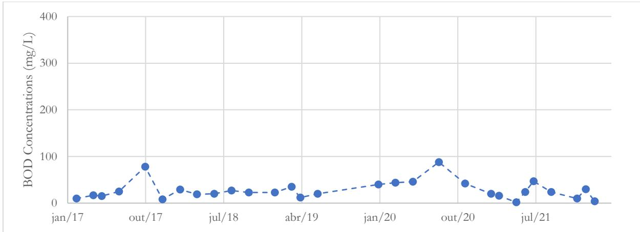
Figure 38 – BOD released by WWTP Quintais do Imperador
