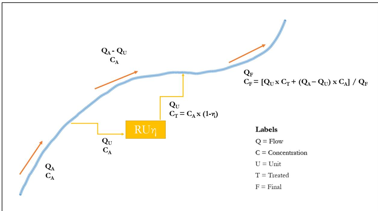
Figure 75 – In situ treatment operation schematic model
