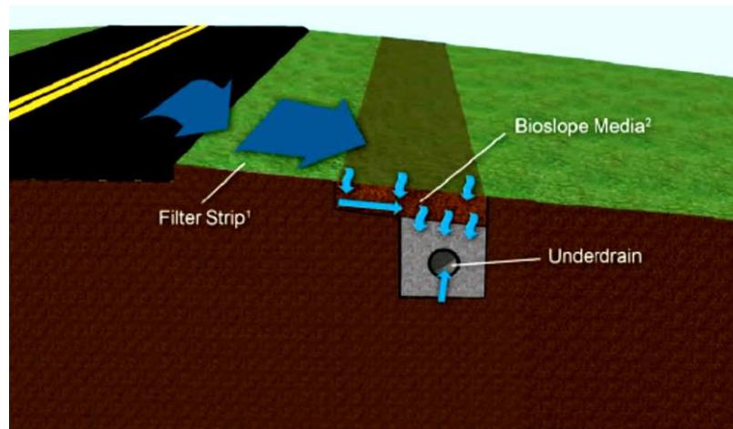
Figure 24 - Bioslope schematic section view
