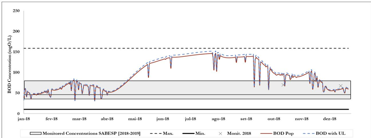
Figure 103 - BOD Concentrations [mg/l] for Jaguaré River Basin - simulated and monitored at Mouth
