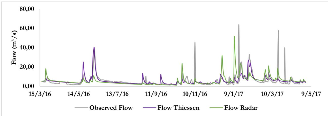
Figure 94 – Comparisons between simulated flow obtained through rainfall from radar (green line) and rainfall from Thiessen's method (purple line)
