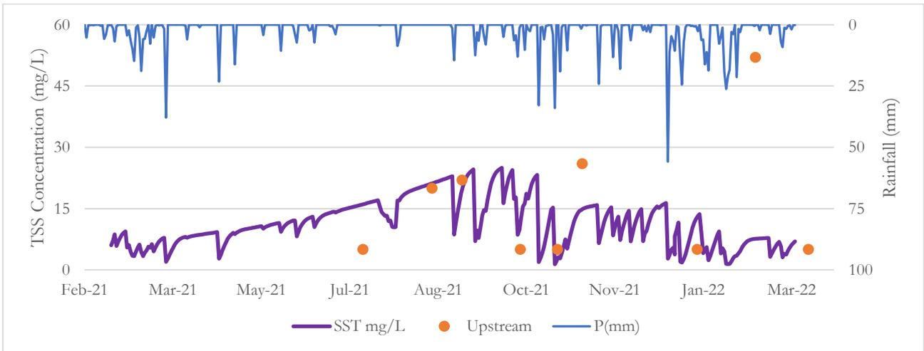
Figure 88 - TSS Concentrations [mg/L] for Hedberg Reservoir - simulated (purple line) and observed (orange dots)
