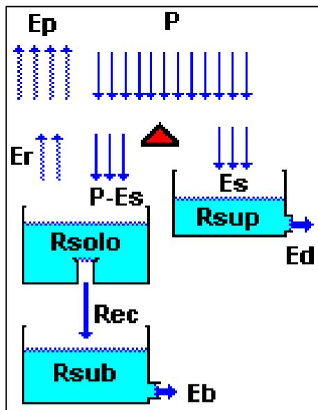
Figure 62 - Illustration of the Daily Flow Forecast Model
