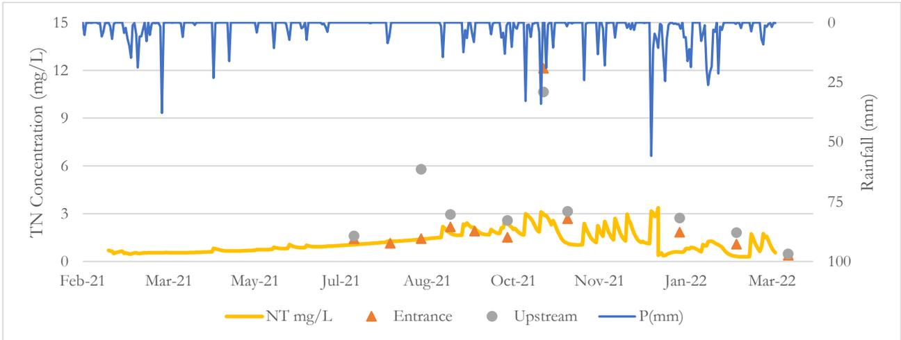
Figure 87 - TN Concentrations [mg/L] for Hedberg Reservoir – simulated (yellow line) and observed (dots)
