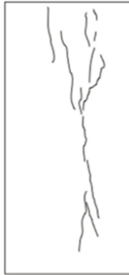
Figure 39 – Schematic image from Nogales (2020) for experimental cracking pattern observed in Schnutgen and Erdem (2001) results
