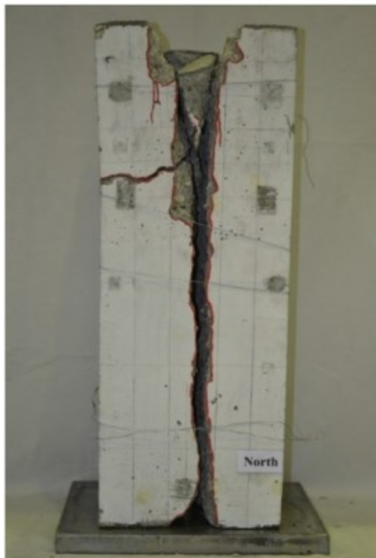
Figure 29 - Experimental cracking pattern in plain concrete sample - Tiberti et al. (2015)
