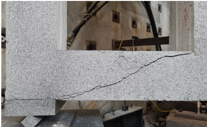
Figure 11 – Photograph of the area of failure in specimen SIIIa upon unloading.
