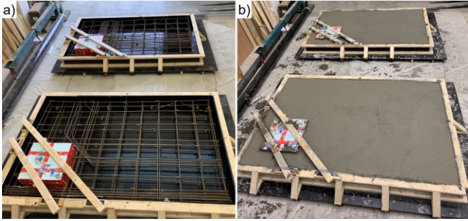
Figure 5 – Specimens fabrication a) before concrete casting b) after concrete casting.
