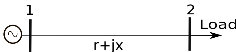
Figure 1 – Two bus system
