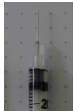
(d) Syringe that does not leak fluid because it contains the attached needle
