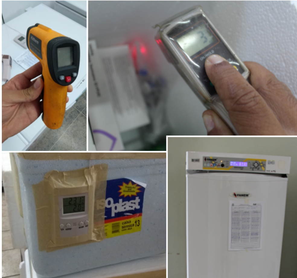
Figure 8: Laser thermometers on the top, digital thermometer on the bottom-left and scientific cooler on the bottom-right.
