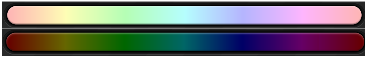
Figure 54 – Color palettes obtained with the HSL color model. The brighter palette (top) was achieved with 95% saturation and 85% on lightness while the bottom darker palette adopted 100% and 20% respectively.
