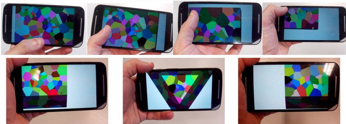
Figure 17 – Mobile navigation. Typical touch operations for translations (top row): initial position, moving sideways, up and down; Intuitive movements for rotations (bottom row): initial position (center), rotating left around the green grain in the corner (left) and right around the same corner (right).
