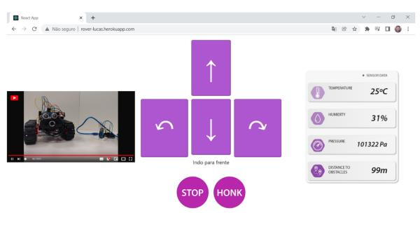
Figure 23 - Web interface of the cyber-physical systems remote lab
