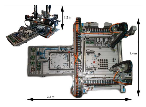
Figure 8 - Schematic representation of the xCPS platform
