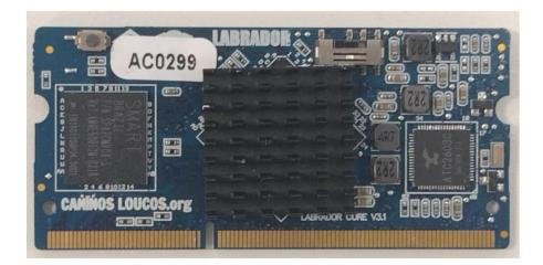
Figure 16 - Core board of the Labrador single board computer
