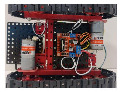
Figure 19 - DC motors and the dual H-bridge motor driver assembled in the smart vehicle
