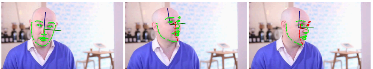
Figure 5-1 Multi-task approach. Simultaneous head pose estimation, facial landmark location and their visibility predictions.
