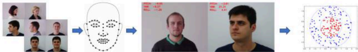
Figure 5-3 Head pose classification process.
