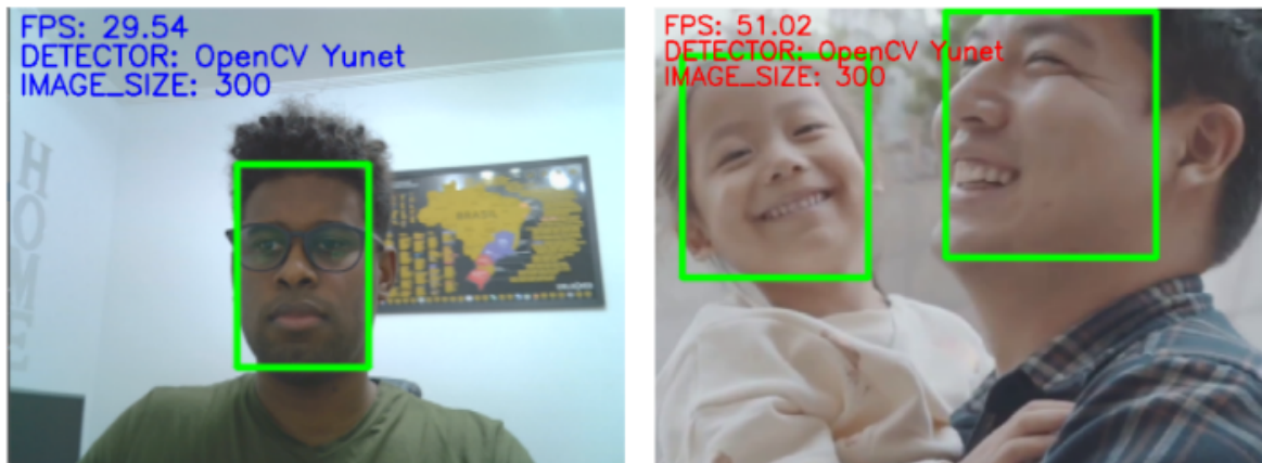
Figure 4-4 Face detection speed running comparison. Left: live webcam video analysis. Right: pre-recorded video analysis.
