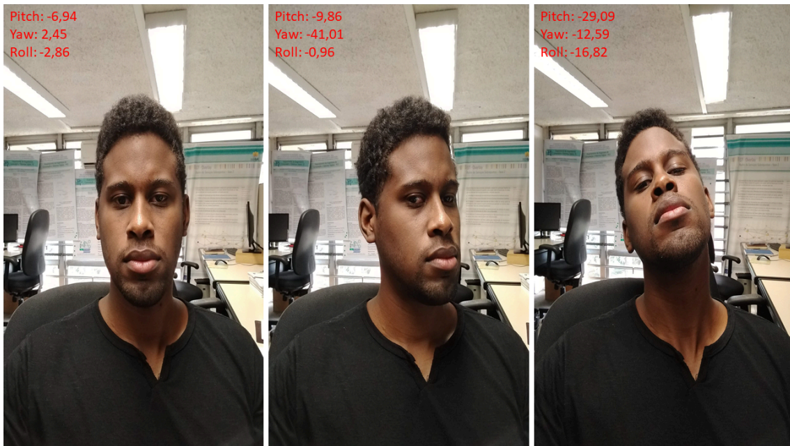
Figure 4-10 Euler angles detection example.
