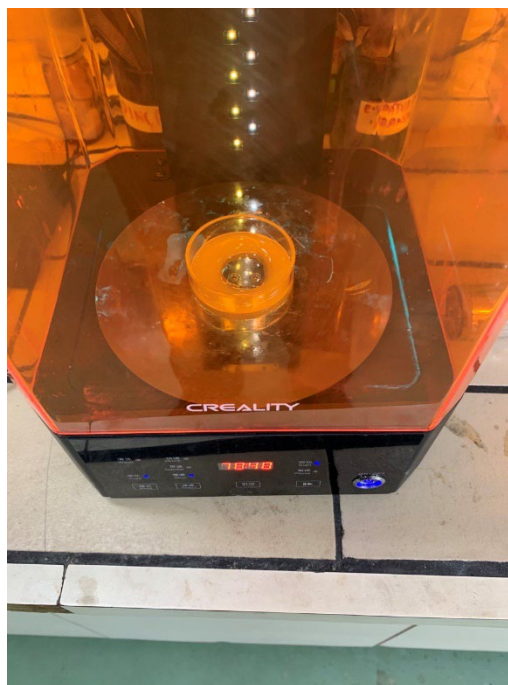
Figure 3. 5 Polymerization initiated by apply UV light
