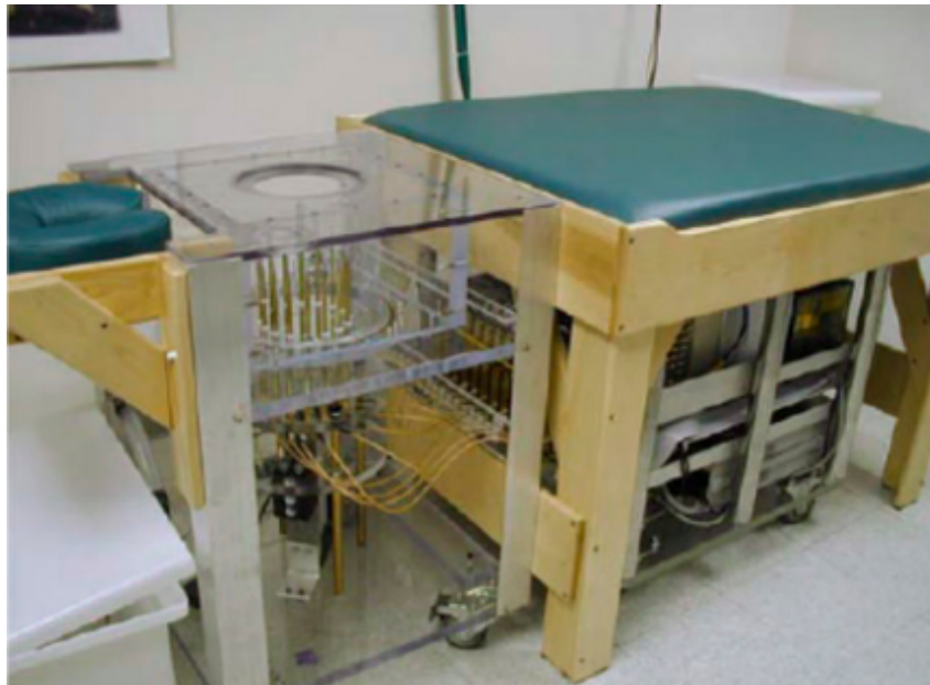
Figure 17 – Photograph of the second-generation MWI prototype made up of a cylindrical array of 16 monopole sensors.
