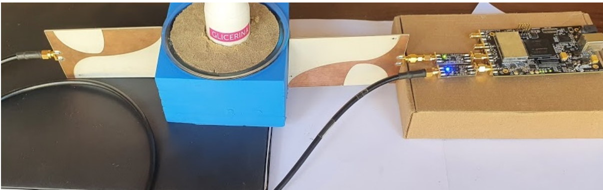
Figure 42 – BladeRF 2.0 coupled with the PA and LNA illuminating the breast phantom through the Vivaldi antennas.
