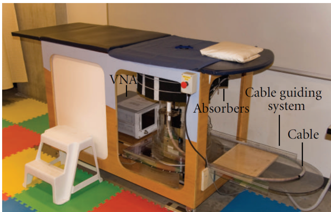
Figure 21 – Photograph of the system composed of the table, one VNA, and cables. Source: (BOURQUI; SILL; FEAR, 2012).
