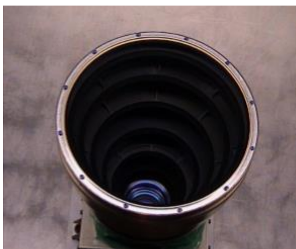
Figura 9 - Foto do “baffle” do SED 16 (EADS SODERN)
