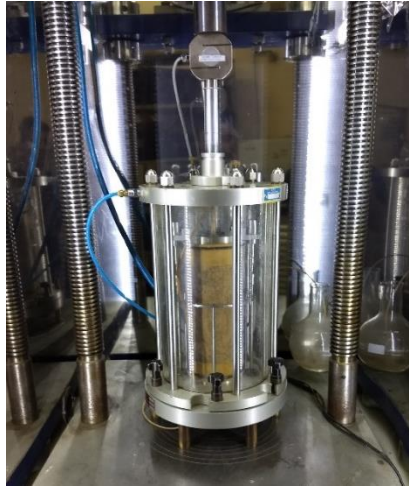
Figure 53 - Specimen during Tx RM test
