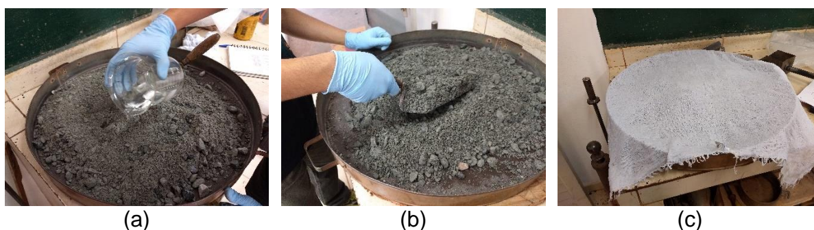
Figure 46 - (a) Moisture correction, (b) homogenization and (c) covering for moisture loss prevention
