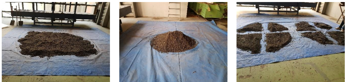
Figure 44 - Quartering process of RAP_2F1H
