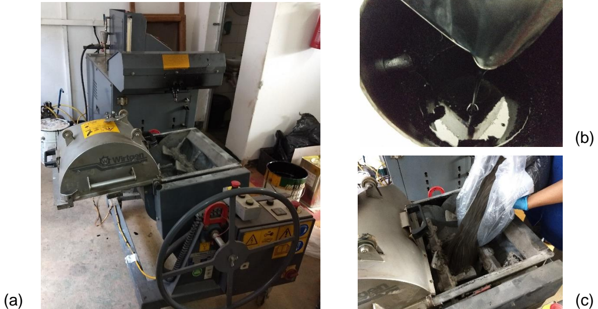
Figure 15 - (a) Wirtgen WLB 10s foaming machine and placement of the (b) binder and (c) aggregates
