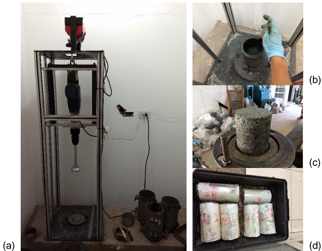
Figure 47 - Compaction stages using (a) a vibratory hammer: (b) material being laid inside the mold, (c) specimen extraction and (d) storage
