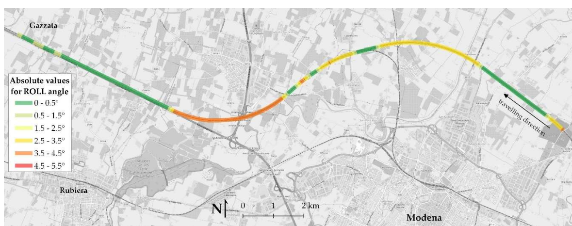
Figure 55 - Map of roll angle (absolute values) versus track geometry for the first day, stretch B
