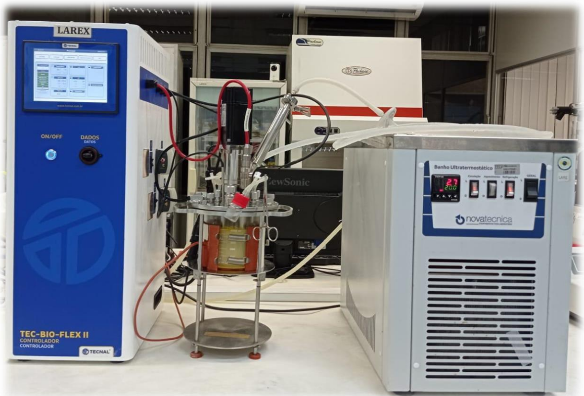
Figure 13 - Fermentation of corn and sugarcane mixed wort in bioreactor
