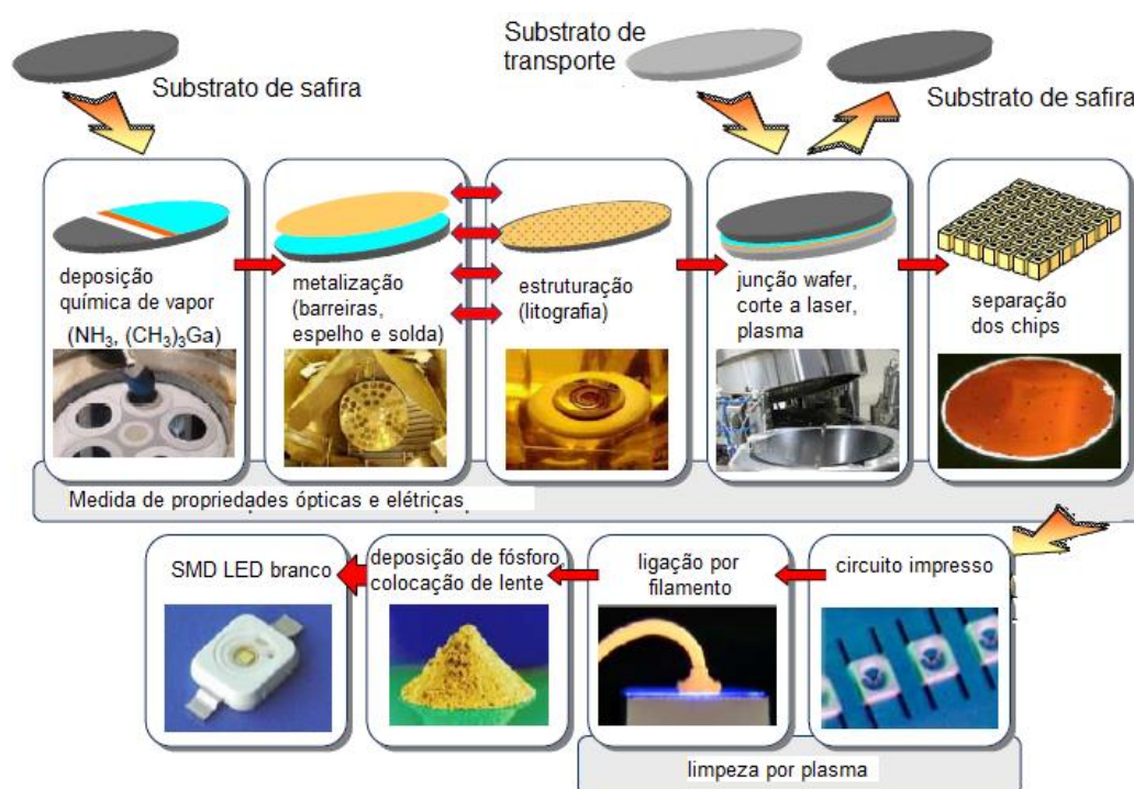
Figura 4 – Processo de manufatura de LED branco (OSRAM OPTO SEMICONDUCTORS e SIEMENS CORPORATE TECHNOLOGY, 2009).
