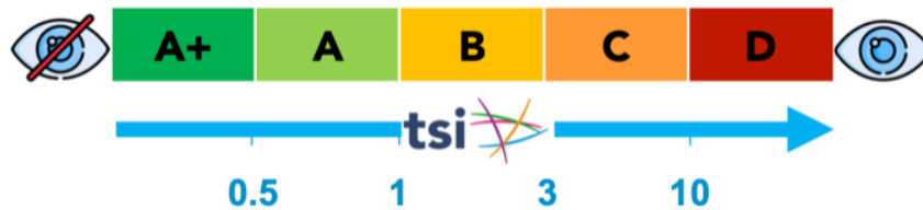
Figure 13 - TSI scale used as stability criteria and correlation to visual observation (Formulacion, 2019).
