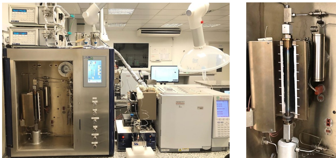
Figure 12 – Microactivity Effi automated reaction system for gas-to-liquid processes.
