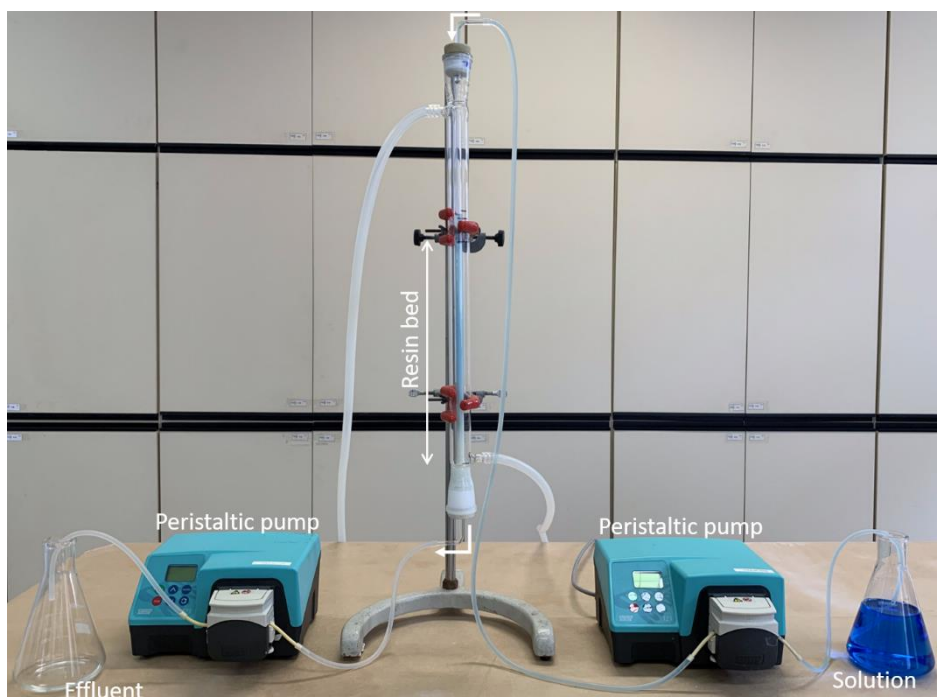
Figure 19. Apparatus used in the fixed bed column experiments.
