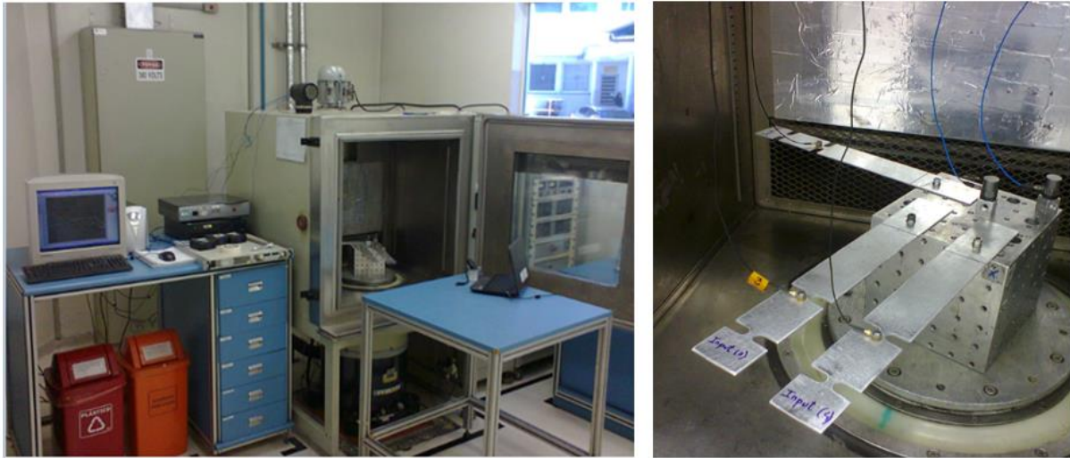
Figure 38 - Hardware used to conduct the vibration test
