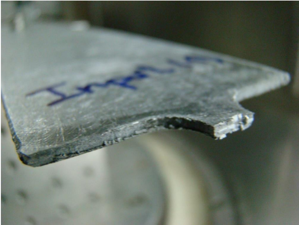
Figure 66 - Sample 2 fracture detail
