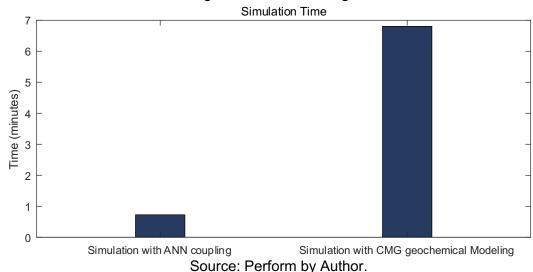
Figure 12: Simulation time comparison between the ANN coupling solution and conventional geochemical modeling.
