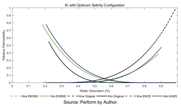
Figure 14: Relative permeability of Engineered Water Optimized versus Normal relative permeability.
