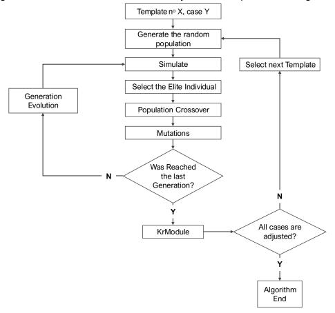
Figure 5: Workflow of Relative Permeability module coupled to FGA algorithm.
