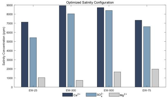
Figure 13: Ionic concentration of water injection obtained by the optimization process.
