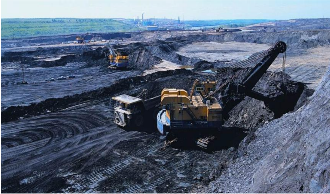
Figure 13 - Modern oil sands mining by 400 tonne truck and cable shovel.
