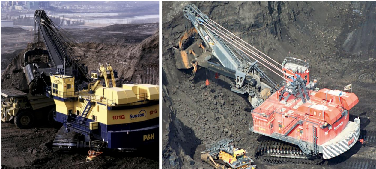
Figure 10 - Electric shovels: Suncor (Left) and Syncrude (Right)
