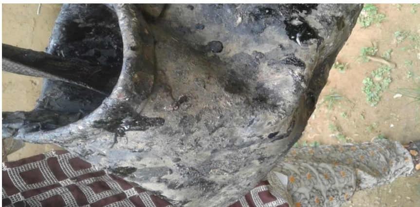
Figure 32 - Water fetcher stained with bitumen seepage
