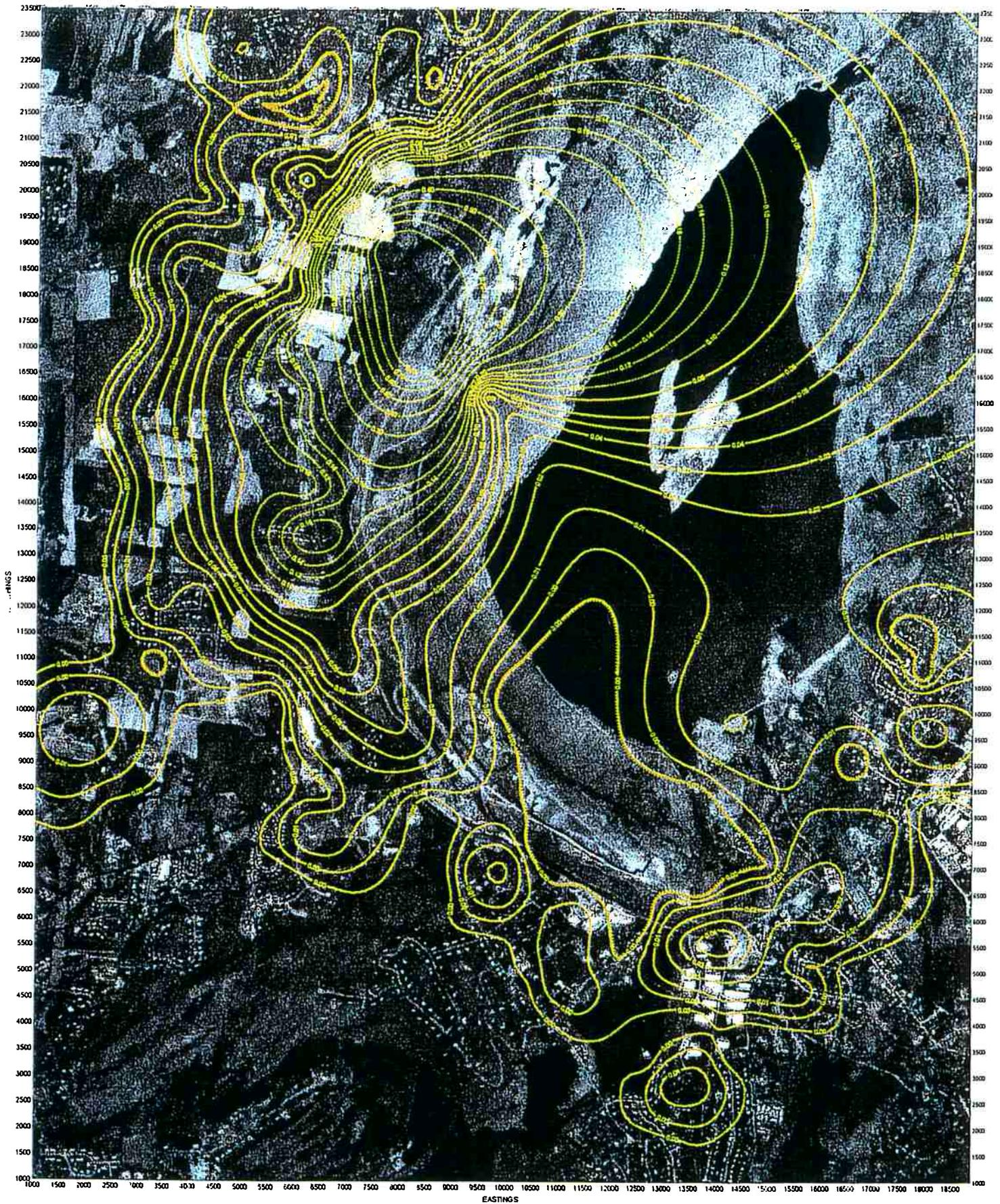
**Iso-Seismic Contour Map of Peak Particle Velocity from the detonation of a single explosive column at a New England Traprock Quarry**
