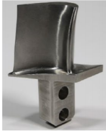
Figure 27 – Turbine blade of \text{Fe}_{25}\text{Al}_{1.5}\text{Ta} alloy, cast and machined. Source: [143]
