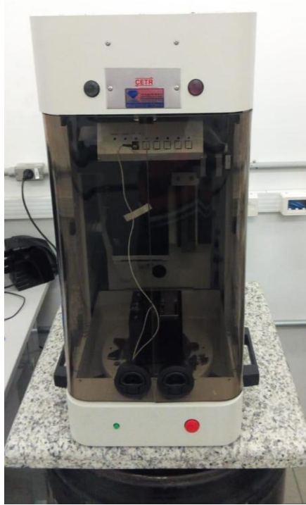
Figure 24: CETR-UMT Multi-Specimen Test System equipment.
