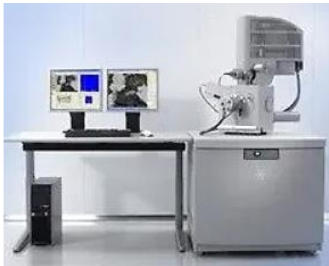
Figure 21: Scanning electron microscope (SEM) with field emission gun - FEG - Inspect F50
