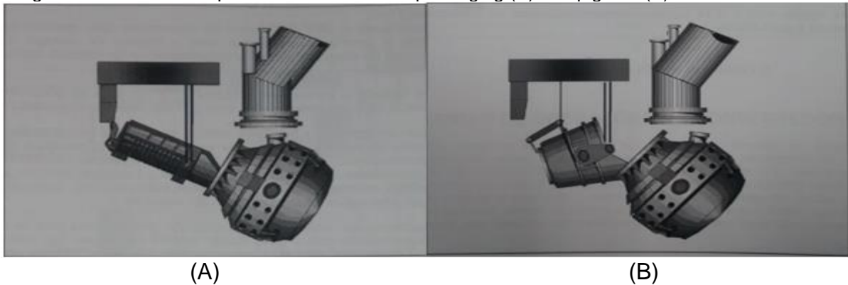
Figure 2 – Schematic representation of the scrap charging (A) and pig iron (B) in the converters LD
