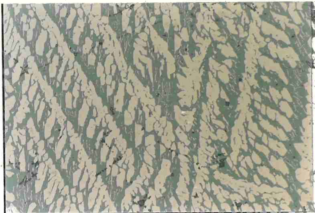
Figura 4.2.11 Microestrutura de liga \text{Nd}_{35}\text{Fe}_{65} tratada a 600^{\circ}\text{C} , mostrando as fases \text{Nd}_2\text{Fe}_{17} e \text{Nd-}\alpha . (400x) (foto C34-7)
