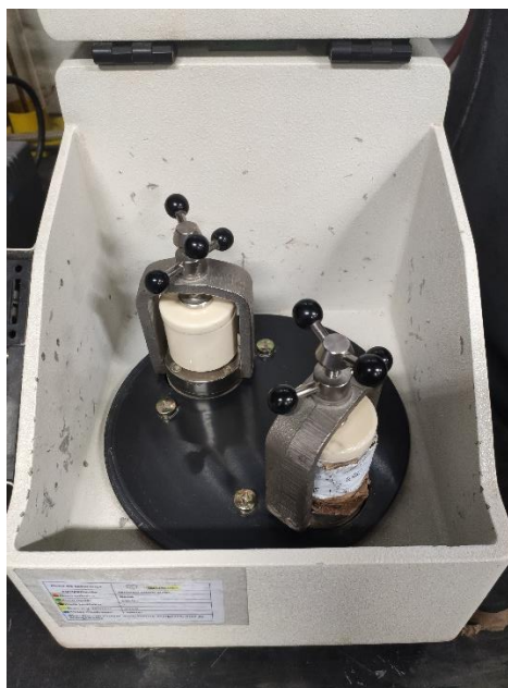
Figura 29 - Moinho Fritsch (planetary micro mil pulverisette 7).
