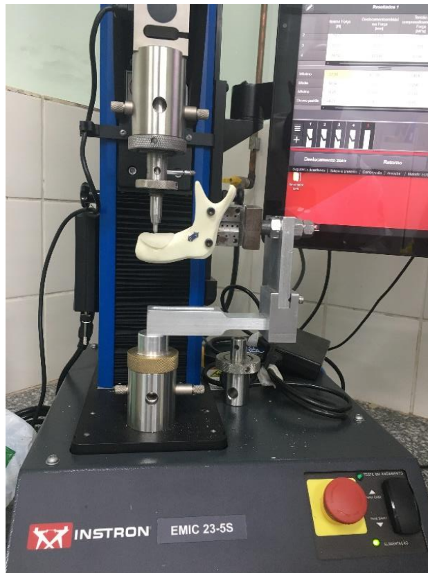
Fig. 5 – The universal testing machine Instron Emic 23-5S
