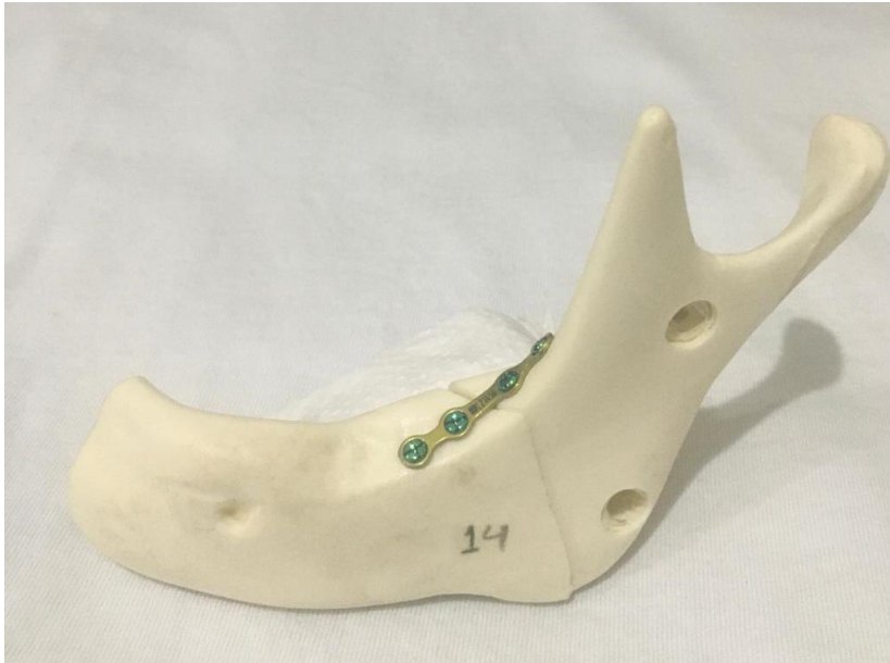
Fig. 3 – Group 1, fixation with a conventional 4-hole titanium miniplate according to Champy principles.
