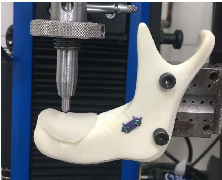
Fig. 7 – The posterior end of the ramus segment fixed to a metallic support that was in turn mounted on the machine of mechanical testing.
