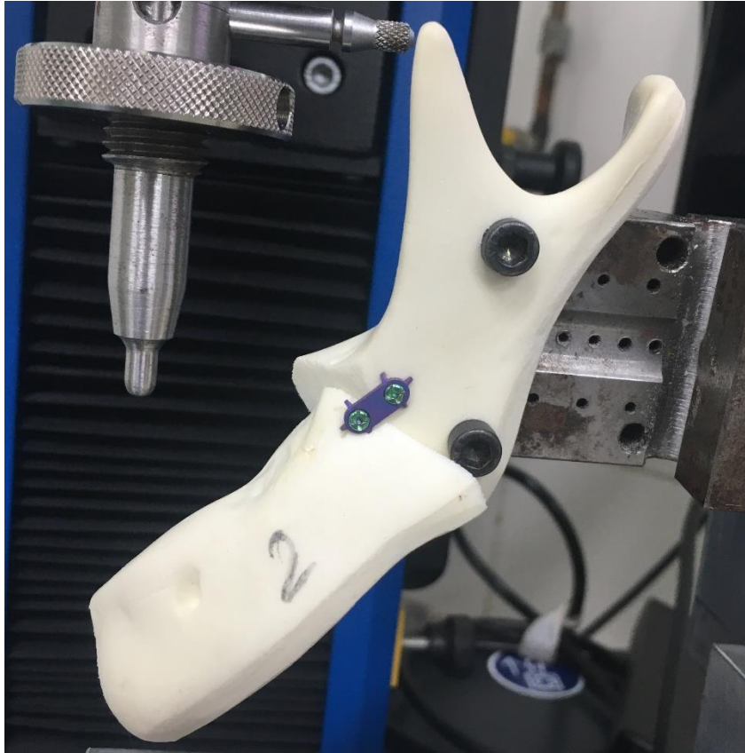
Fig. 10 - A vertical progressive force applied until a fixation failure or a fracture in the hemimandible was observed.
