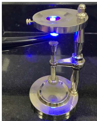
Figure 5 - Device used to position the light source below the ceramic slice.
