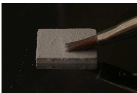
Figure 2 - Manual application of \text{nTiO}_2 alcohol/acetone mixtures.
