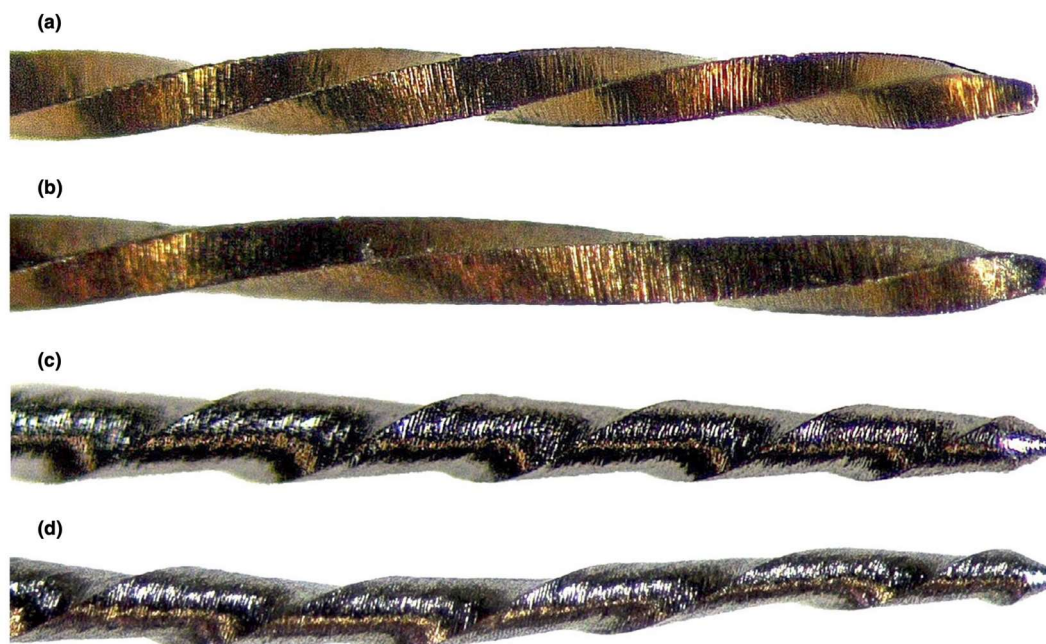
Figure 1 Stereomicroscopy view of instrument surfaces before and after glide path preparation. (a) Intact WaveOne Gold Glider. (b) WaveOne Gold Glider showing deformation of helical structure, after glide path preparation. (c) Intact R-Pilot. (d) R-Pilot showing deformation of structure, after glide path preparation.
