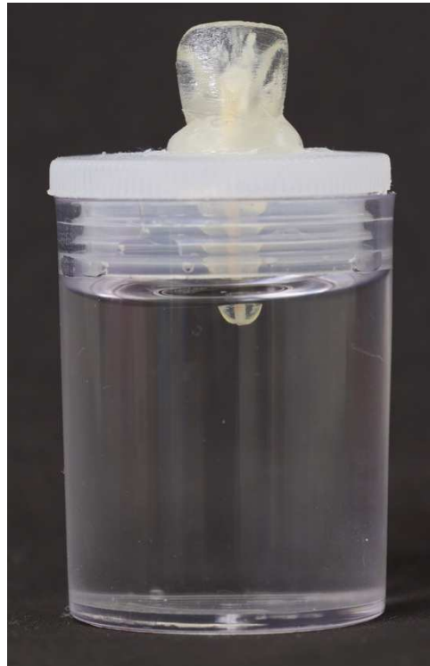
Fig. 1 Root canal of prototype tooth filled with root apex in constant contact with moisture
